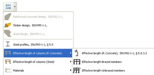
In the appearing windows for computing the effective lengths of columns in braced or unbraced frames, you input the basic frame dimensions and section properties.
